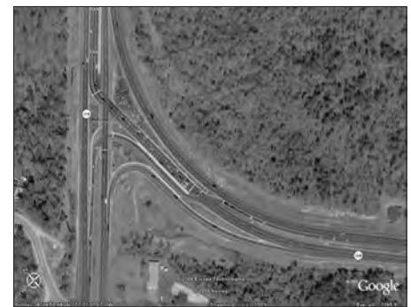
A continuous flow intersection (CFI) in Accokeek, MD, built in 2000. This CFI reduced average delay by 40-50%. (Photo: Courtesy of Google Pro)
